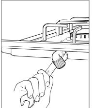
If installation is to be carried out using a flexible connector (to BS669), then the following points must be adhered to:
